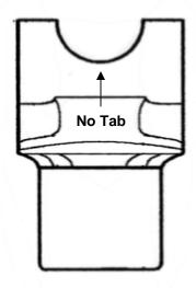
Inside Lock up Width - This type yoke uses the C-Clips on the UJ cap to lock the UJ into place. C-Clips must be used on this type of yoke or the UJ caps will come out.
