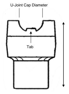
Measure UJ width from inside edges of tabs - where the UJ will actually fit
