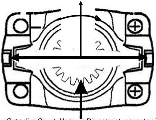
Get spline Count- Measure Diameter at deepest point across to exact other side at deepest point.
